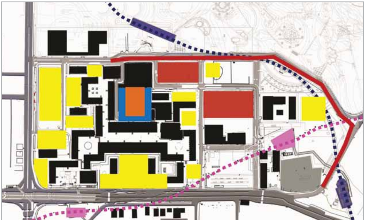
Orange Multi-Level Car Park Yellow At Grade Car Park Blue Goods Vehicle Park Red Informal Parking
